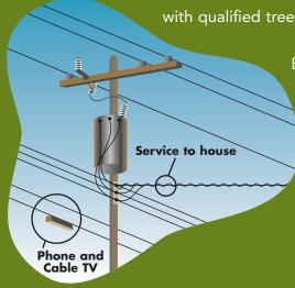
Electric lines usually are located at the top of the pole, farthest from the ground. Cable TV and telephone lines run closer to the ground, below power lines.
